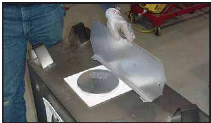
Figure 9.2 Rotate the top heat shield to the vertical position as shown above. The heat shield must remain in the vertical position.
